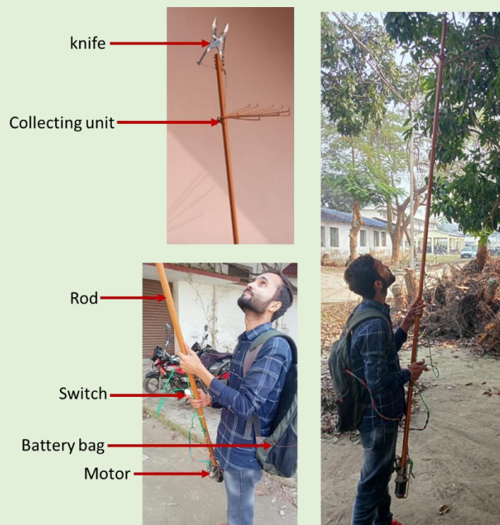
Fig. 2. Overall view of final model of litchi harvester with collecting mechanism
