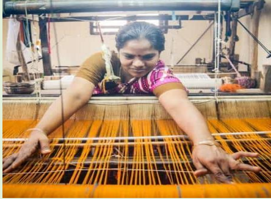
Fig 4: Weaving Process Using Banana Yarns
