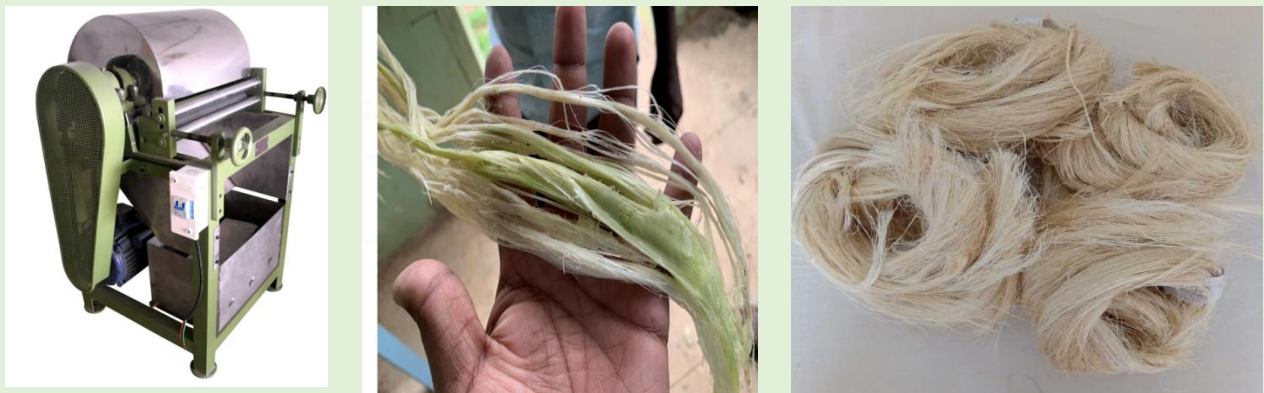
Fig. 2. Steps from pseudo stem collection to fiber extraction and product development
